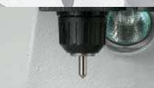
4. Micrometric ring for setting up (0,02")
